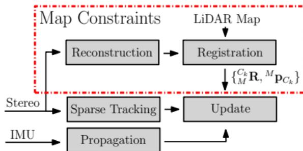
**Figure 2:** Data flow and proposed map constraint generation.
