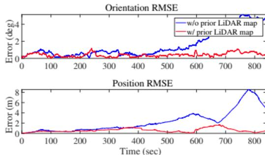
**Figure 6:** Orientation and position RMSE for the standard MSCKF and map-aided MSCKF with prior LiDAR map noises of  $\sigma = 0.03m$ ).
