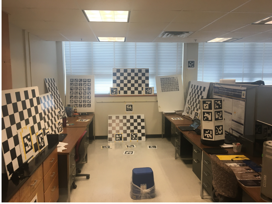
Figure 2: Proof-of-concept indoor experiment setup for the proposed aided INS with point and plane features. ArUco makers [31] are placed in the workspace to serve as planar point features and thus to create point-on-plane constraints.
