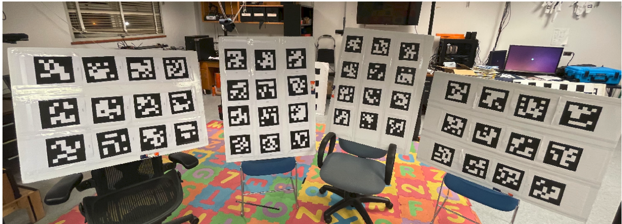
Figure 7: ArUco tags for stable visual feature tracking.
