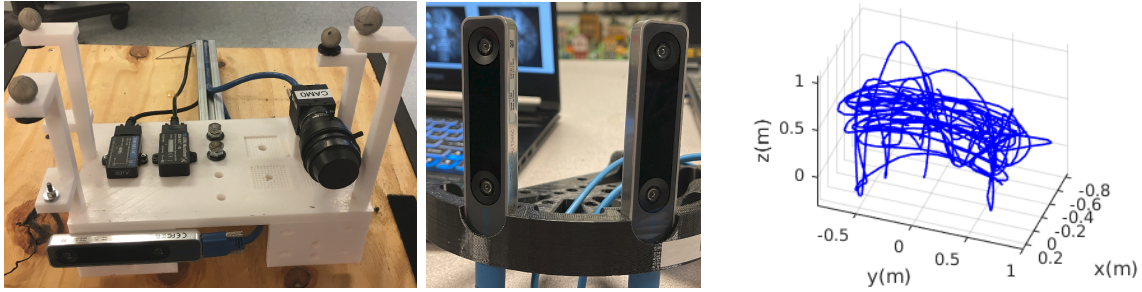
Figure 6: The self-assembled sensor rigs in real-world experiments. Left: VI-rigs containing 2 Mircostrain IMUs, 1 BlackFly camera and 1 IntelRealsense T265 tacking camera. Right: T265-rigs containing 2 IntelRealsense T265 tracking cameras.
