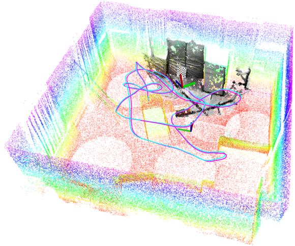
Fig. 1. The proposed visual-inertial localization system with the prior LiDAR map constraints runs on the EurocMav dataset [9]. The prior LiDAR map is colored by height, while the groundtruth and estimated trajectory are plotted in cyan and pink, respectively. A semi-dense pointcloud reconstructed from a series of keyframes is also shown in black.
