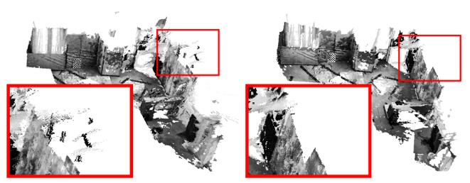
Fig. 3. Visual semi-dense reconstruction without depth refinement (left) has high levels of noise on walls of the room. By contrast, the visual semi-dense reconstruction *with* depth refinement (right) exhibits lower amounts of noise along the boundary (see picture inset). These pointclouds are a small subset of the EurocMav V1\_02\_medium sequence [36].
