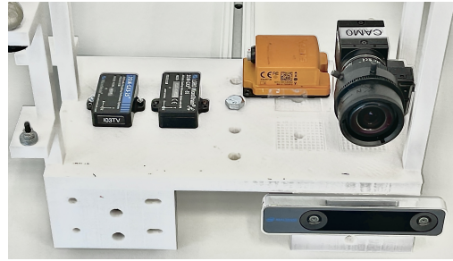
Fig. 12: Visual-Inertial Sensor Rig contains a MS-GX5-25 IMU, MS-GX5-35, Xsens MTi 100, FLIR Blackfly camera and RealSense T265 tracking camera (containing an integrated IMU and a fisheye stereo camera).
