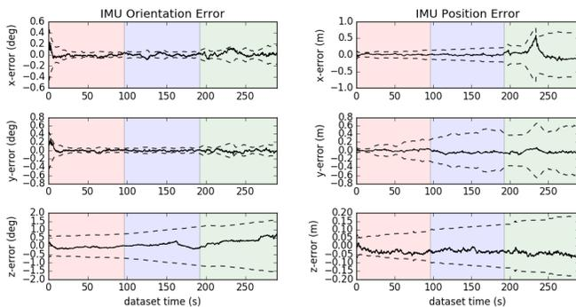
Figure 6: The orientation and position of the proposed MIMC-VINS in the presence of sensor dropouts. The segments of the trajectory are broken into three parts: in the first (red), all three components are operational. In the second (blue), the first component pair has failed. In the final (green), the second component pair has also failed, leaving only one IMU-camera pair operational. Despite these failures, redundant sensing allows for continuous and accurate estimation of the platform.
