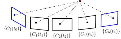
Figure 2: Illustration of how asynchronous multi-camera measurements are collected. We have cloned at the base camera imaging times:  $\{C_b(t_0)\}, \{C_b(t_4)\}$  (blue). A series of measurements between these times from non-base cameras  $C_1$  and  $C_2$  are received. We can interpolate to these pose times using the base camera cloned poses.
