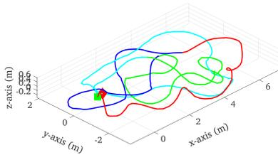
Figure 9: The trajectory estimates of the proposed MIMC-VINS on multicam\_1 dataset in the presence of sensor dropouts. Red section has 3 camera and 2 IMU, blue has 2 camera and 2 IMU, green has 2 camera and 1 IMU, and cyan has 1 camera and 1 IMU.
