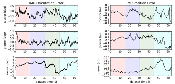
Figure 10: The pose estimation errors of the proposed MIMC-VINS on multicam\_1 dataset in the presence of sensor dropouts. The first camera is dropped out at 15 seconds, the first IMU at 30 seconds, and the second camera at 45 seconds into the dataset.
