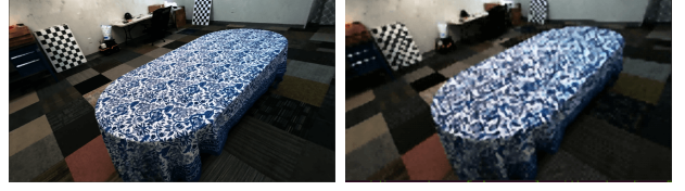
Fig. 2: Example rendered images for testing matching methods. Left : Rendered image with resolution 424 \times 240 . Right : Rendered image with 141 \times 80 resolution and up-scaled to 424 \times 240 with FSRCNN [52].
