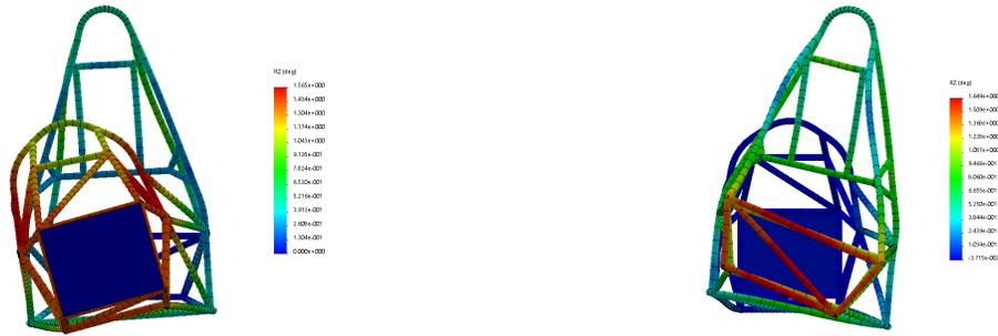
Figure 16: Iteration 5 FEA of the torsional rigidity of the front suspension box (left) and back suspension box (right).
