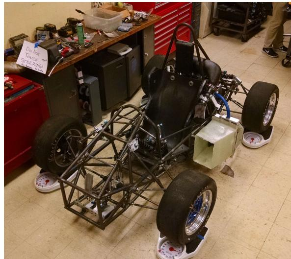
Figure 39: (Left) The jig used to test the torsional rigidity where the rear end is fixed and the front would pivot about a point. A moment was applied to observe the displacement of the chassis which could then be related to the torsional rigidity calculation. (Right) The setup used to calculate the weight distribution of the car. Note that the experimental value recorded was performed with a driver.
