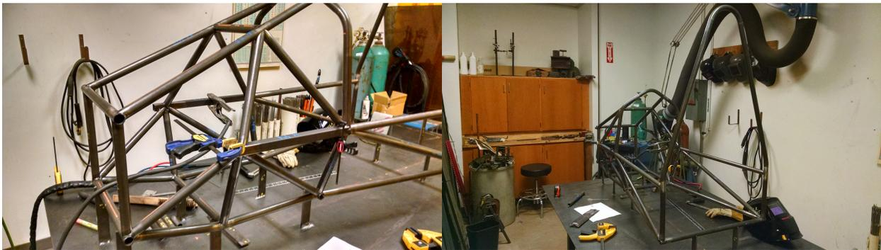
Figure 36: The front suspension box and front bulk head supports tacked.
