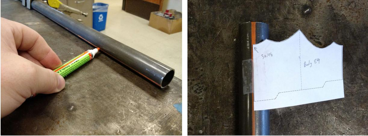
Figure 67: Drawing a continuous centerline down the pipe (left) and then the applied paper cutout aligned to the centerline on the desired pipe (right)
