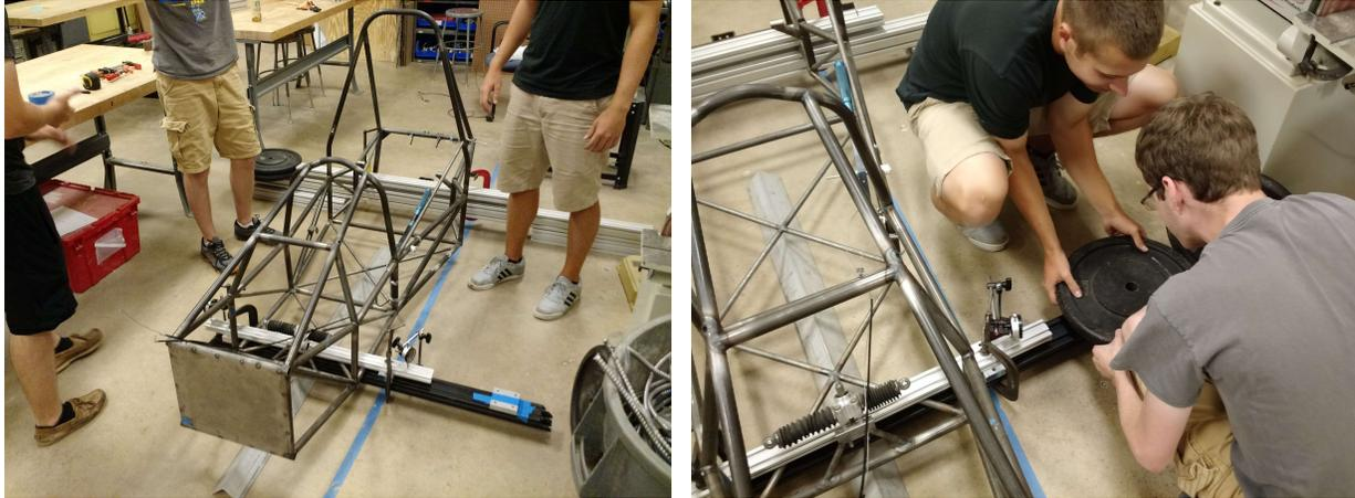
Figure 52: The total mounting platform (left) and the team putting weights on the cantilever beam (right)
