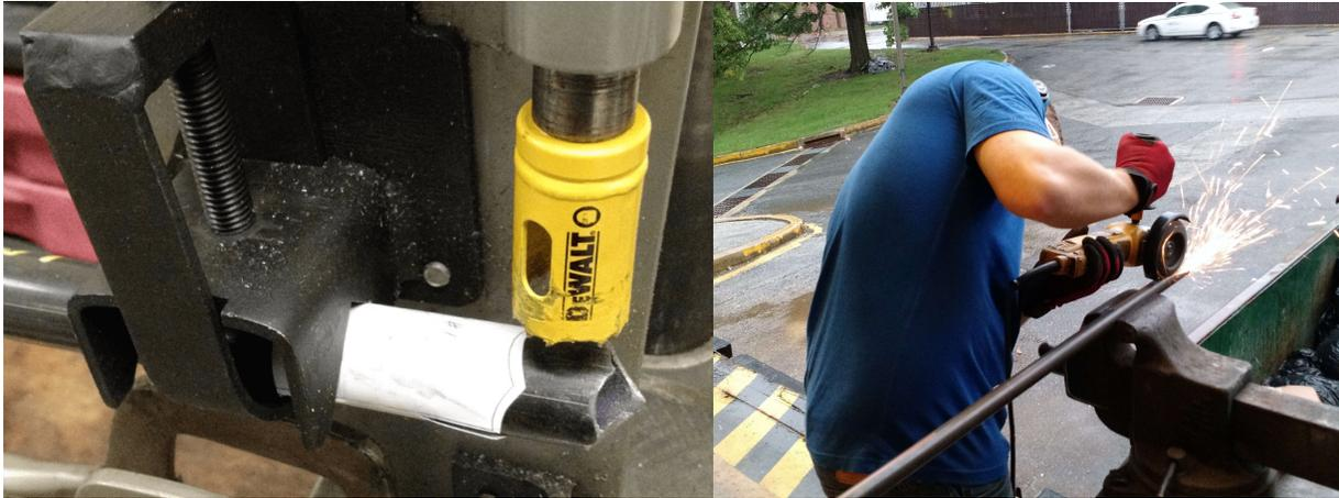
Figure 69: Tube being ready to notch (note that the paper is removed before notching) and a pipe being ground to the paint outline outside the FSAE room.
