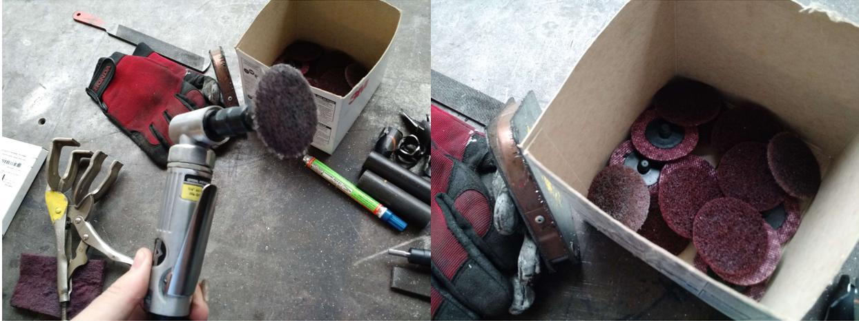
Figure 34: Above is the air tool used to prepare tubes for welding, and the removal of rust from pipes. 2 inch Aluminum Oxide Quick Change disks with a Type R attachment are used ordered from MSC.
