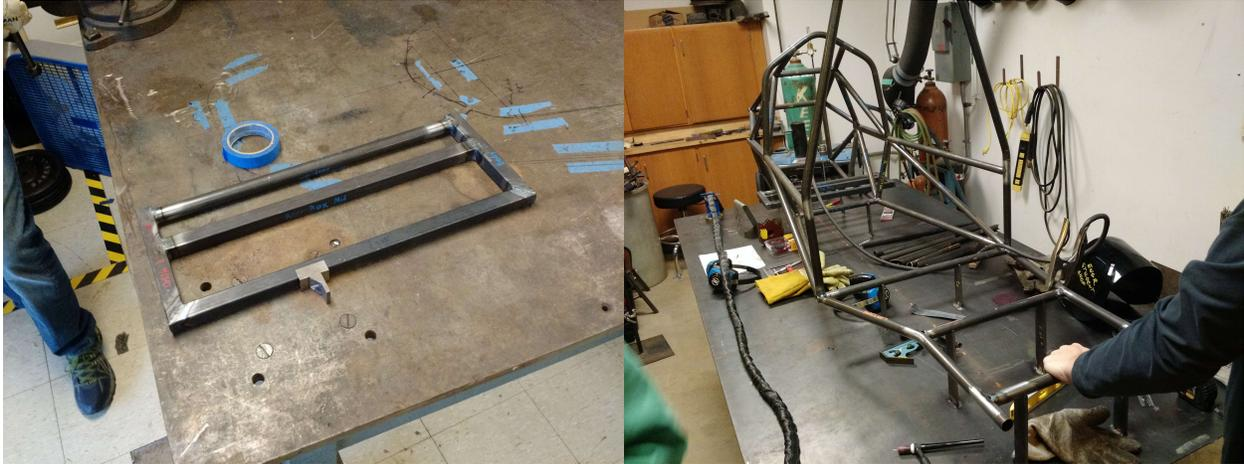
Figure 37: The top of the rear suspension box fully squared and welded (left). Initial tacks on the rear suspension box (right). The welding jig ensured accuracy was maintained.
