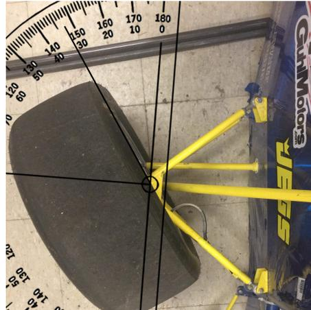
Figure 57: Geometry of a fixed back wheel and a front wheel turning at angle  $\alpha$  (left), and a photo of the angle on the 2014 chassis at max steer angle of 33 degrees (right)
