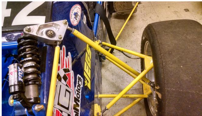
Figure 45: The forward suspension of the 2014 University of Delaware FSAE car.
