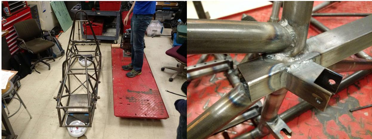
Figure 40: Finished chassis getting weighed, and an example finished weld on the front suspension box.
