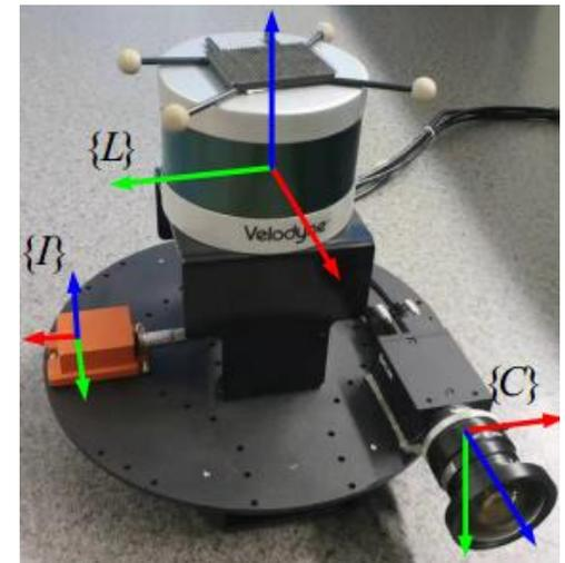
Fig. Sensor setup with a 3D LiDAR, IMU and a monocular camera.
