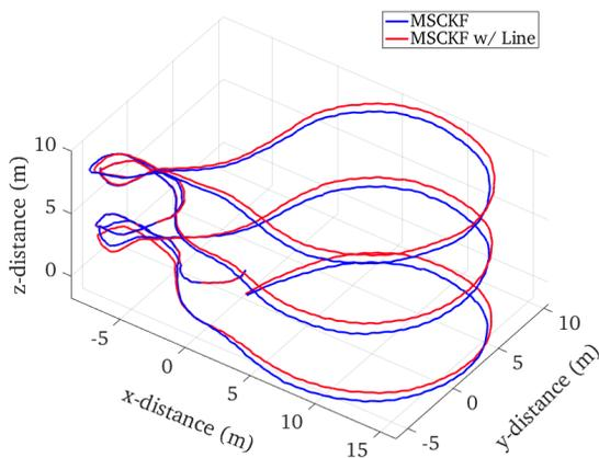
Fig. 4: Trajectory of the 223 meter long University of Delaware Gore dataset spanning three floors.
