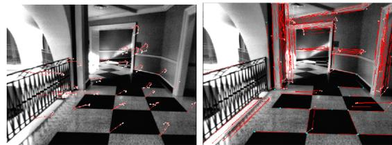
Fig. 5: Example tracking on the University of Delaware Gore dataset for both point features (left) and line tracks (right). A history of tracks has been overlaid for each point/line in the image.
